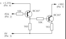
The above circuit can be used to indicate both positive and negative polarity, by illuminating either the + or - segment on the meter.
