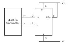
Measuring a current loop. The meter power supply should be isolated from the 4-20mA transmitter power supply
