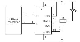
Using an external LED as a high alarm and a switch to acknowledge the alarm (to stop it flashing)
