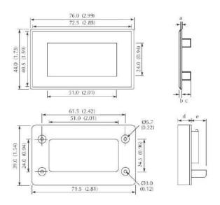
Panel cut-out 72 x 40 (2.83 x 1.57) Maximum panel thickness 3mm (0.12).
