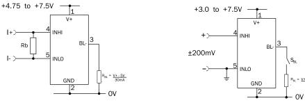
Measuring a single ended input voltage Measuring a current from a circuit which is referenced to a split supply, i.e. the input voltage and the meter's power supply share the same OV rail. Ensure solder link LCOM is open.
