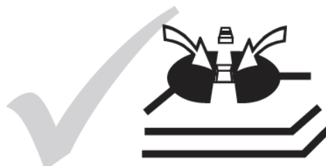
Fig. 9.6 How to cut PCB links
