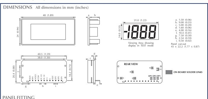
Fit the bezel to the front of the panel and then locate the meter into the bezel from behind. Alternatively the meter and bezel may be assembled before fitting into the front of the panel but care must be taken not to use excessive force. Finally fit the window into the front of the bezel.
