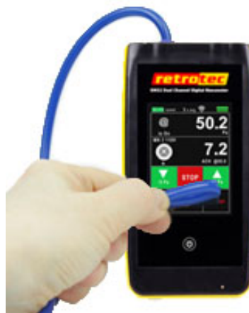
Figure 67: Errors in pressure reading from a pinched tube.
