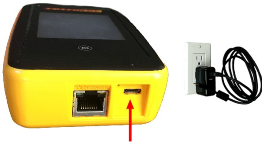
Figure 4: DM32 charging port
