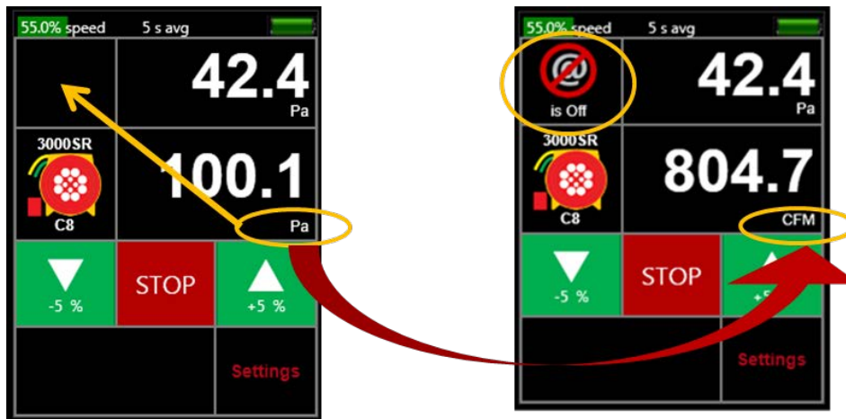
Figure 27: [@ Pressure] is not available when Pressure is the Result on Channel B
