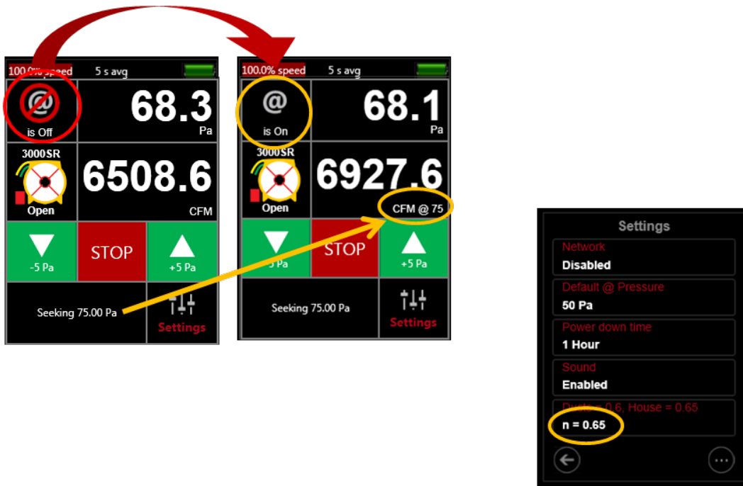
Figure 29: [@ Pressure] extrapolates to the target pressure when a pressure is set
