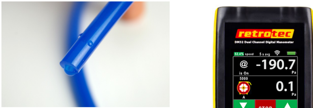
Figure 68: Water in the reference tube (left); high fixed pressure due to water (right).
