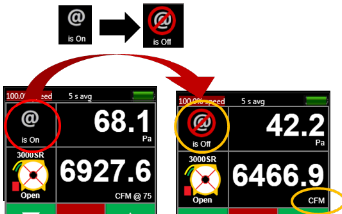
Figure 32: Turn [@ Pressure] off, leaves fan running
