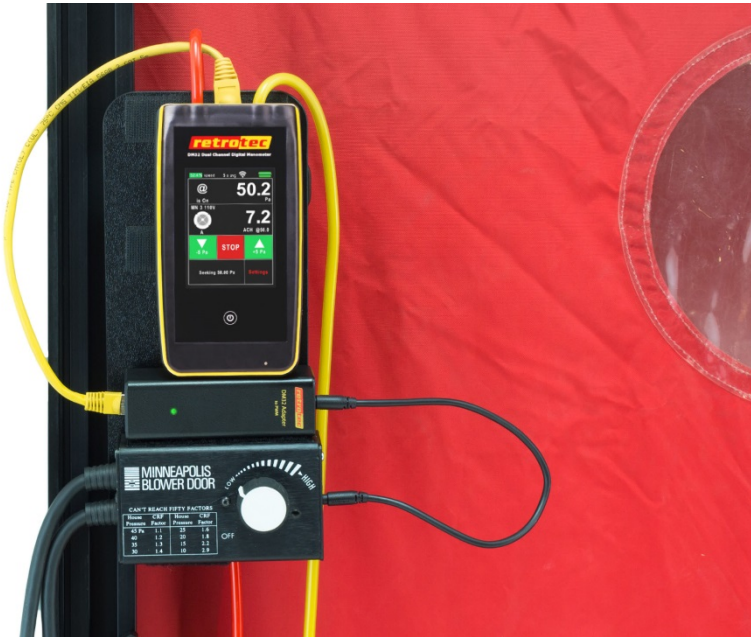
Figure 12: Control a TEC fan using the gauge and Fan Speed Control Adapter (part FN275, produced by Retrotec)
