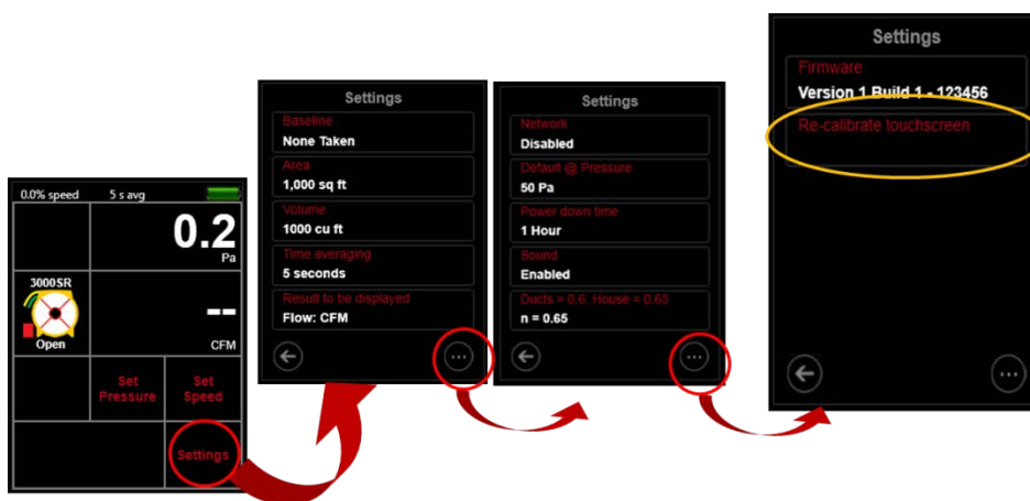
Figure 50: Start the re-calibrate touchscreen process from the third Settings screen
