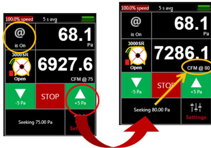
Figure 30: Jogging pressure while using [@ Pressure] changes target and @ pressure label
