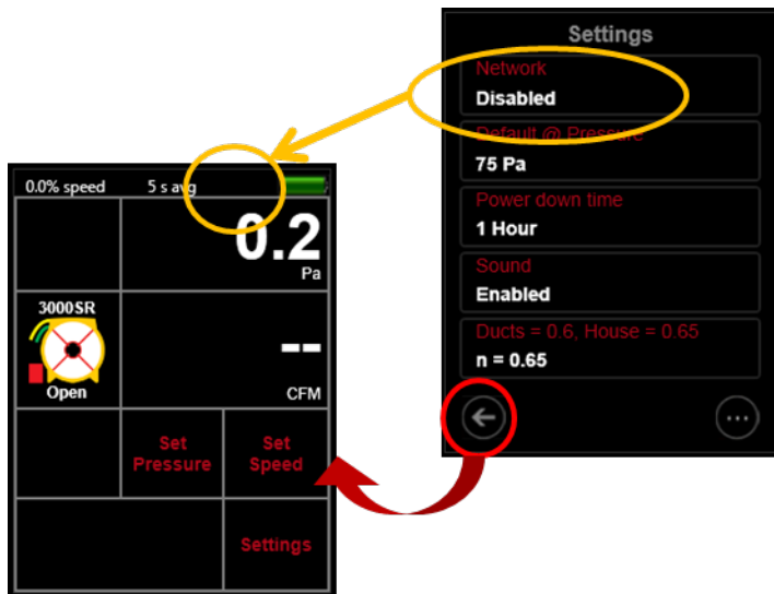
Figure 63: Disable [Network] connection if using USB connection to a computer
