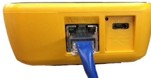
Figure 53: Ethernet cable goes into "Network" connector on gauge for a "Wired" Network
