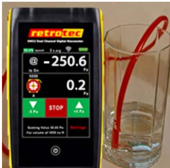
Figure 71: The gauge displaying a negative pressure (-250.6 Pa).
