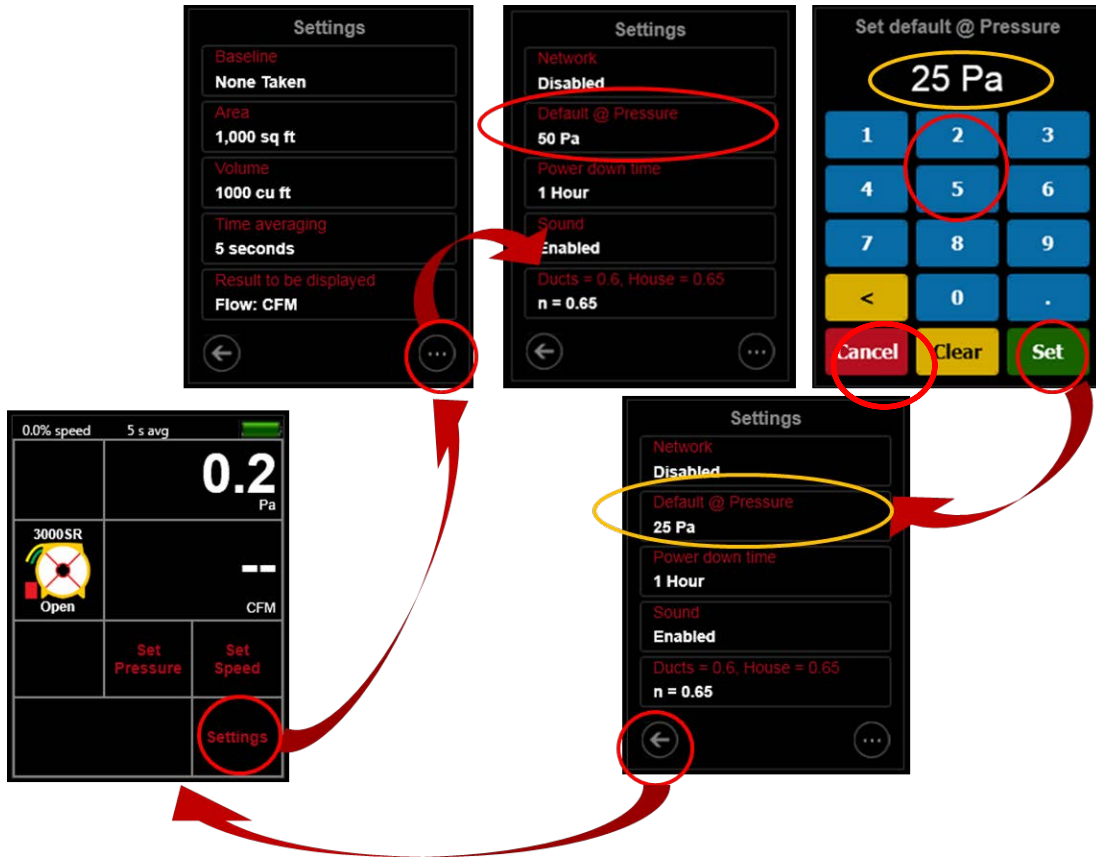
Figure 43: Set the default @ pressure to be used as extrapolation pressure during set speed operation
