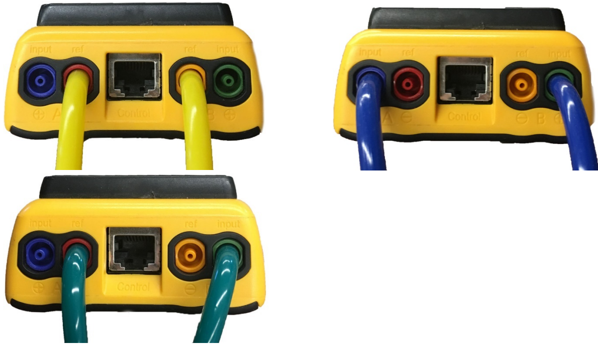
Figure 64: Yellow tube between Channel A & B. Blue tube check of positive ports. Green from negative to positive ports.
