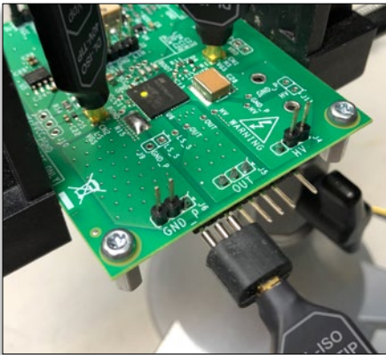
DL-ISO measuring V_{gs} (MMCX) and V_{ds} (header pins) signals
