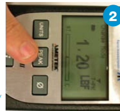
Select Units of Measure Select the UNITS key to specify the units of measure you want displayed.
