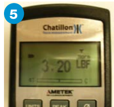
Observe Load Read the force result from the display. If you select the PEAK key after you complete your test, the DFX II will display the maximum (Peak) load that was achieved during the test.
