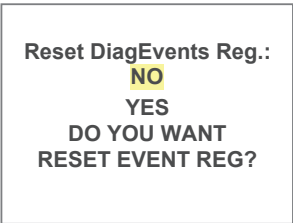
Figure 51: Resetting Diagnostic Events Register
