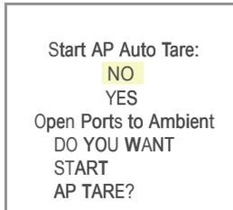
**Figure 39:** Start AP (Absolute Pressure) Sensor Tare
