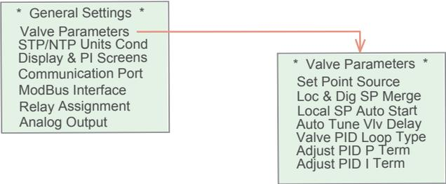
**Figure 14:** General Settings and Valve Parameters Menu Selections
