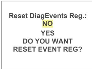
**Figure 51:** Resetting Diagnostic Events Register
