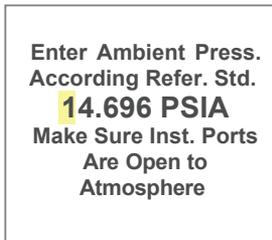
**Figure 40:** Entering Ambient Pressure from Reference Standard
