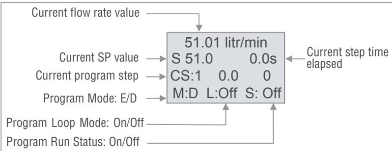
**Figure 35:** Instrument PI Screen #7 with PSP parameters
