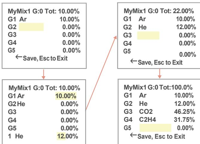
**Figure 26:** Mixture with 4 Components Ready to be Saved
