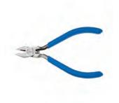
These 4-Inch Klein Tools Midget Electronics Diagonal Cutting Pliers have a semi-flush design to cut nickel ribbon wire. The nose tip is 1/32-Inch and the tip cutting knife is 3/16-Inch for precision in tight areas. Finally the pliers are forged from US steel and have induction hardened cutting knives and a hotriveted joint for a long lasting smooth action.
