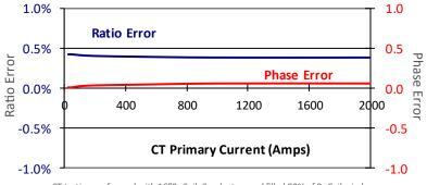
CT testing performed with 16"RoCoil. Conductor used filled 90% of RoCoil window.
