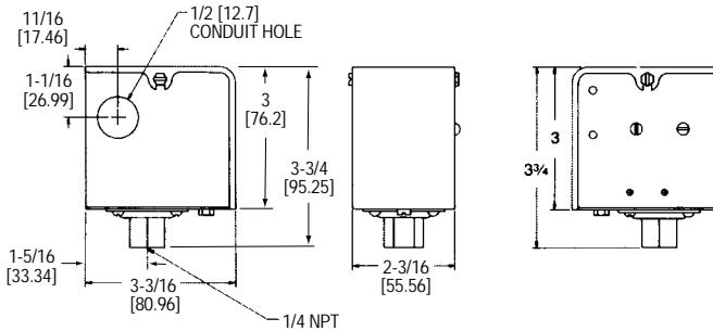
**The Series CS Low Cost Diaphragm Pressure Switch** is ideal for instrument panels, small compressors and general industrial applications. Visible set point and easy-to-wire SPDT snap switch reduce installation time. This switch operates in any position and is vibration resistant.
