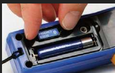
Attach to enable Bluetooth® wireless technology
