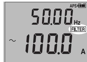
**Frequency characteristics when the filter function is enabled**
