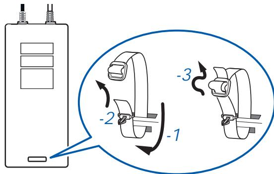
3 Attach the strap buckle to the instrument and connect it to the clip that you attached to the P2000 with the strap.
