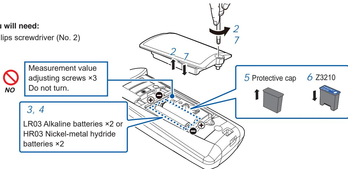
**NO** Do not turn any screws except the battery cover screw.
