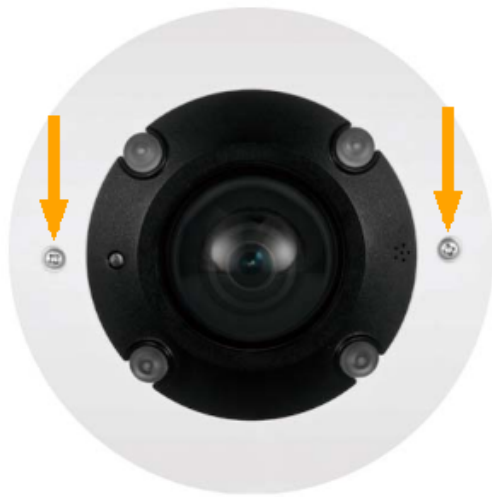
Screws Securing Cover to Base
