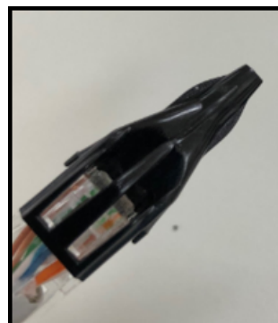
RJ45 Insertion Tool Attached to Terminated Ethernet Cable
