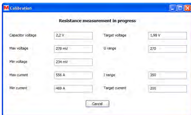
Figure 8.7.3 Resistance measurement progress window
