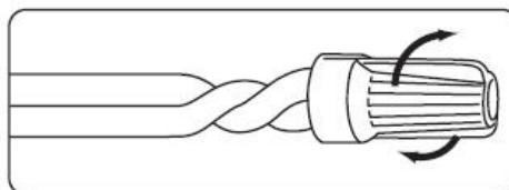
Use only on Copper to Copper (Cu/Cu) wire combinations.
