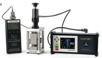
Adhesion testers include everything needed for testing: Adhesion Tester, built-in rechargeable NiMH battery with charger, dollies, abrasive pad, cutting tool, glue with mixing sticks and palettes, cotton swabs, USB cable, PosiSoft Software, instruction booklet, shoulder strap (AT-A only), Certificate of Calibration traceable to NIST, two-year warranty, and sturdy, lightweight carrying case
