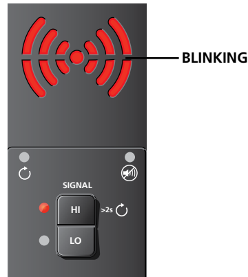
Figure 4.12b: Transmitter indicator showing signal in Loop mode
