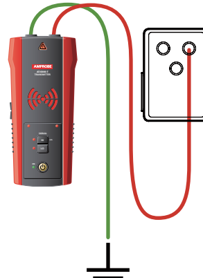
Figure 3.2b: Separate ground connection (Preferred)
