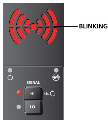
Figure 3.1b: Transmitter indicator showing signal in HIGH mode
