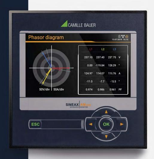
The SINEAX AM-SERIES devices are compact instruments to measure and monitor in heavy current grids. They excel in display quality and intuitive operation. The devices provide a wide range of functionalities which may even be extended by optional components. They are connected to the process environment by communication interfaces, via digital I/Os, analog outputs or relays.
