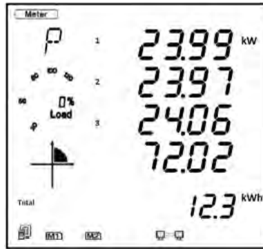
Figure 3-7 - Three-Phase Power Page
