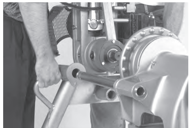
Figure 4 – Sliding Roll Groover Onto Support Arms
