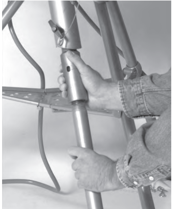
Figure 6 – Adjusting Legs to Level Groover
