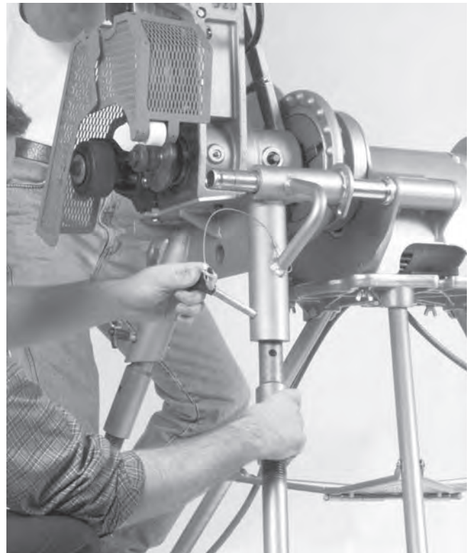
Figure 23 – Removing Legs From Base
