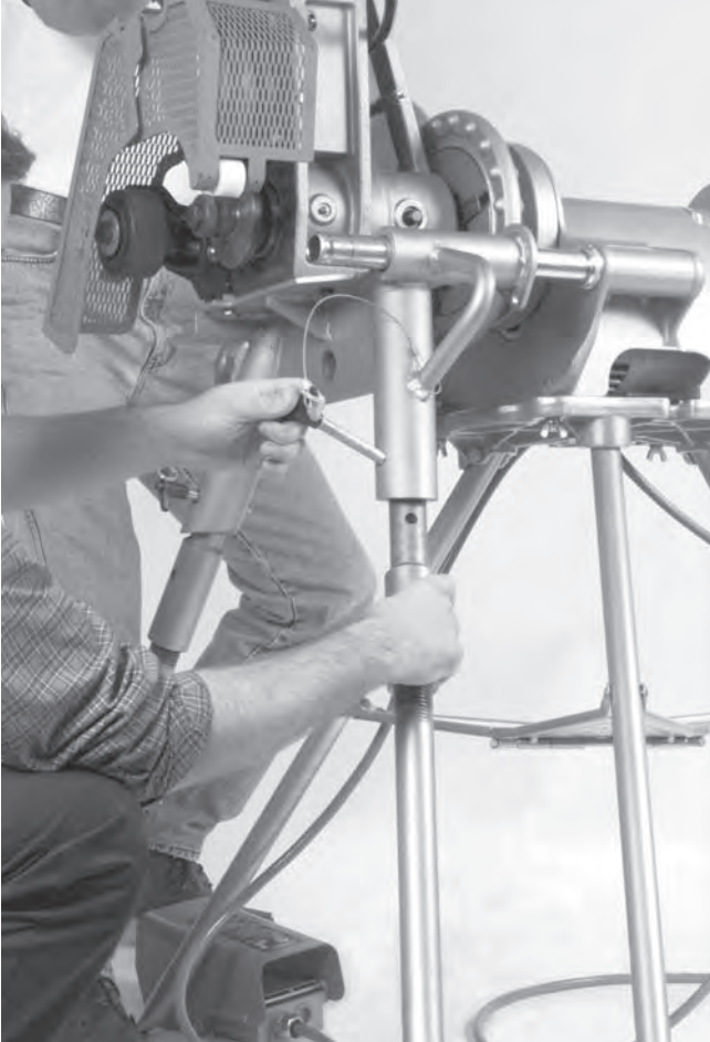
Figure 5 – Installing Legs Into the Groover Base
