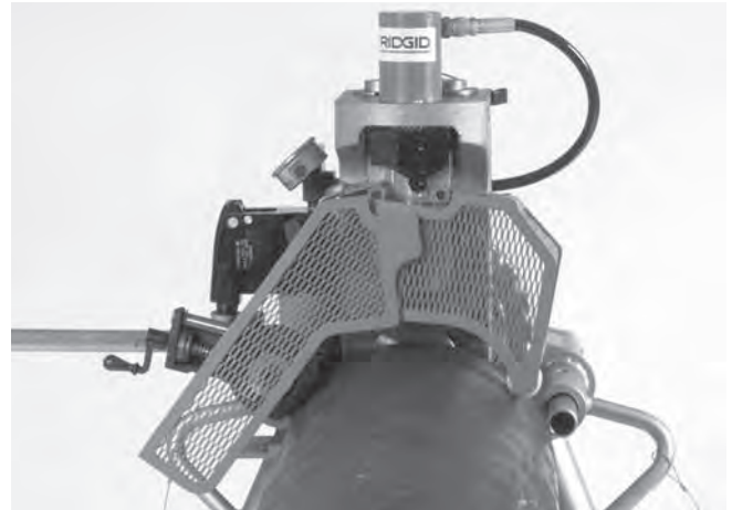
Figure 14 – Guards in the Operating Position
