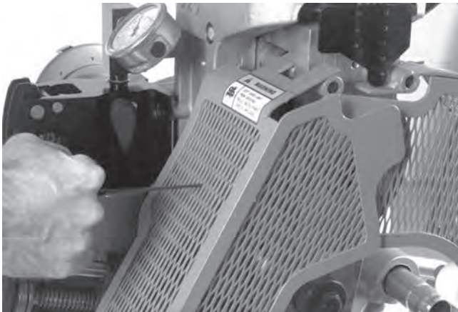
Figure 18 – Loosening Set Screw In Upper Roll Housing
