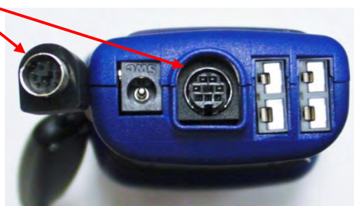
“D” Shaped mini-DIN connector
