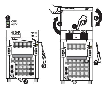
To maintain the full cooling performance, clean the condenser (C) from time to time.
