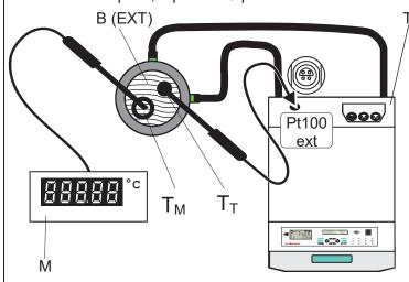
M = Temperature measuring instrument with temperature sensor
