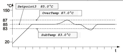
(i) The warning functions are only triggered when the actual bath temperature, after start from the "OFF" or "rOFF" mode, lies within the set limits for 3 seconds.
