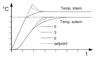
During selftuning, the control parameters Xp, Tn and Tv of a controlled system are automatically determined and stored. Depending on the controlled system, time for tuning can be unequally longer. This controller layout allows protection of sensitive objects requiring temperature application.
