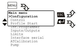
(i) If the electronic module is not fitted, the item >inputs/outputs< will be missing in the menu.
