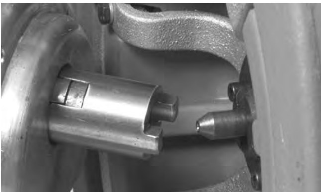
Figure 15 – K-3800 Drum with K-6200 Adapters
