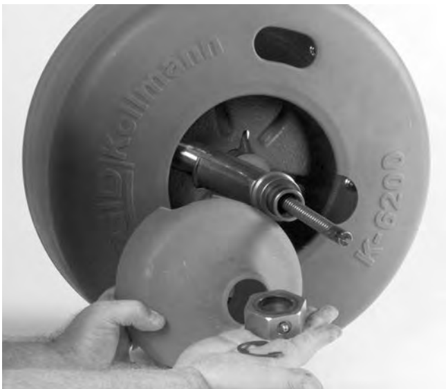
Figure 13 – Remove Retaining Ring and Inner Drum
