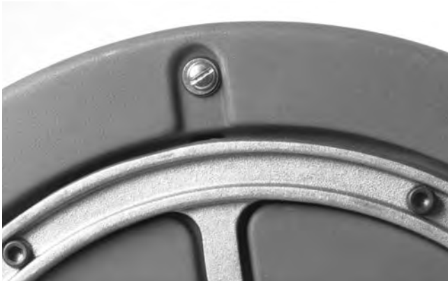
Figure 10 – Drum Drain Hole
