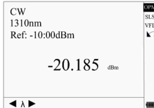
Figure 4-10. Optical Power Meter
