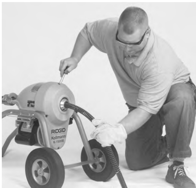
Figure 6 – Proper Operating Position
