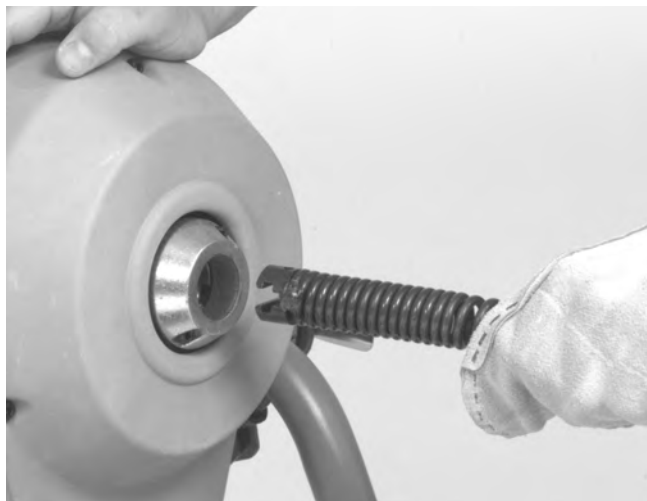
Figure 4 – Inserting Cable Into Front Of Machine
