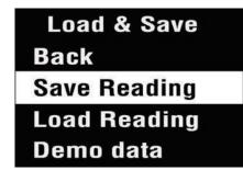
Selecting **Save Reading** opens a screen that allows the user to choose from one of 10 Block No.
