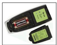
Care must be taken when the batteries are changed. Make sure the gasket is properly seated when reinstalling the battery door otherwise the IP67 rating will be compromised.
