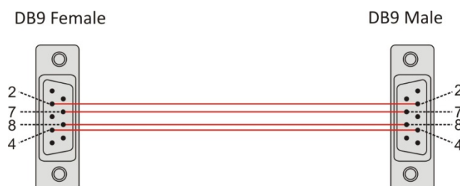
Figure 112 Building an extension cable
