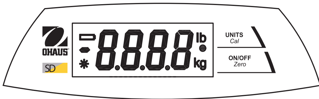
Figure 5. Indicator Panel Controls.
