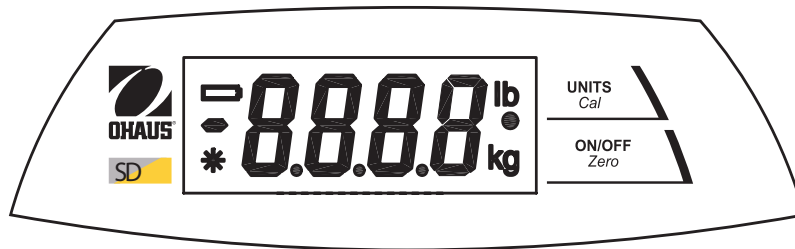
Figure 5. Indicator Panel Controls.
