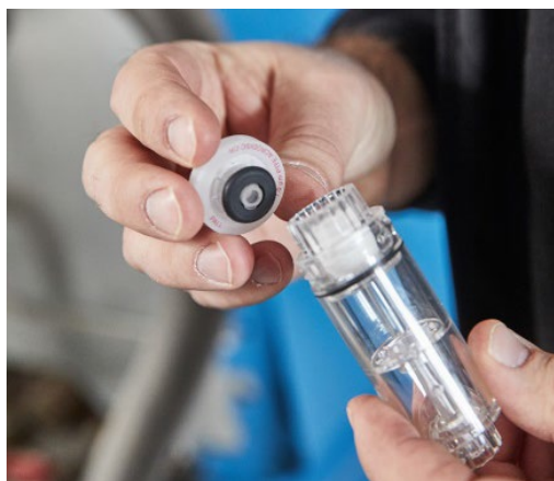
Fig. 46: Filter holder with water stop filter.
