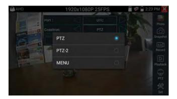
To use coaxial PTZ control with the AHD camera, no parameter settings are needed.
