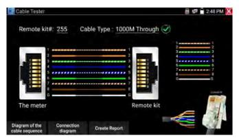
Test LAN cable or telephone cable.
