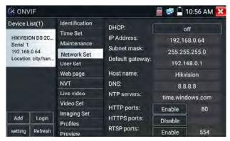
When using the network video input, the tester supports resolutions up to 1080p, the input image remains clear after it is enlarged. This is helpful to installers to ensure the IP camera's video coverage and determine the IP camera's install site.
