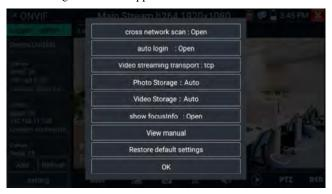
**Across network segments scan:** After opening this function, Rapid ONVIF function can scan across network segments to scan camera's IP.
