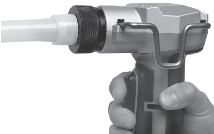
Figure 7B – Tube Expansion Complete, Tube End Flush With Expander Head Shoulder
