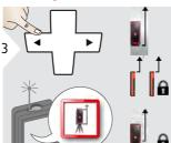
Distance is measured from the rear of the device (standard setting).
