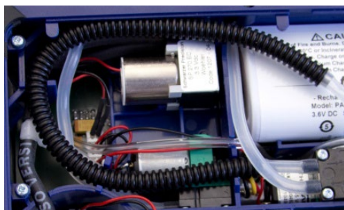
Fig. 79: Corrugated tube, correctly positioned
