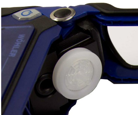
Fig. 72: Water stop filter
