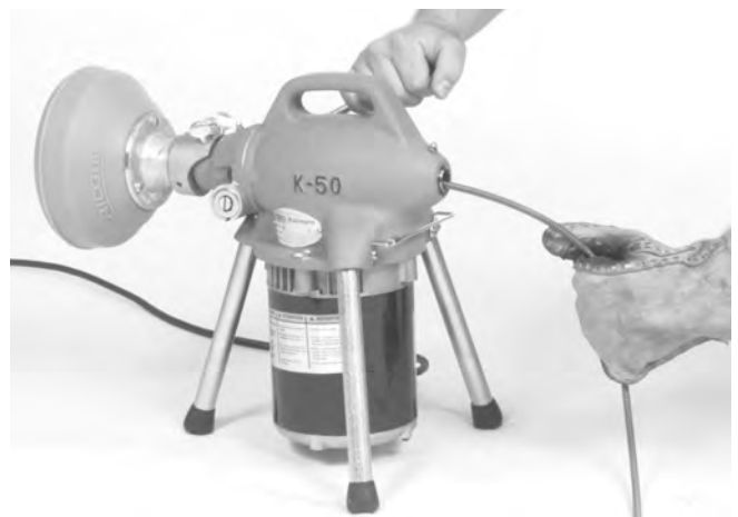
Figure 5 – Cable Adapter Attachment
