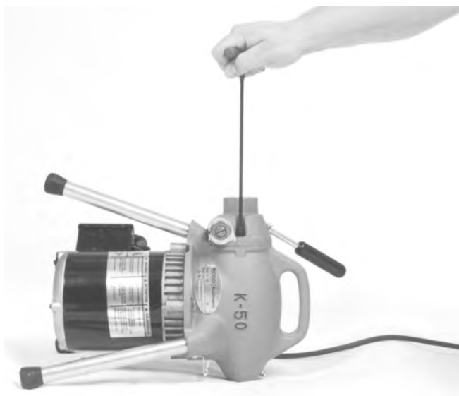
Figure 10 – Retrait des vis Allen
