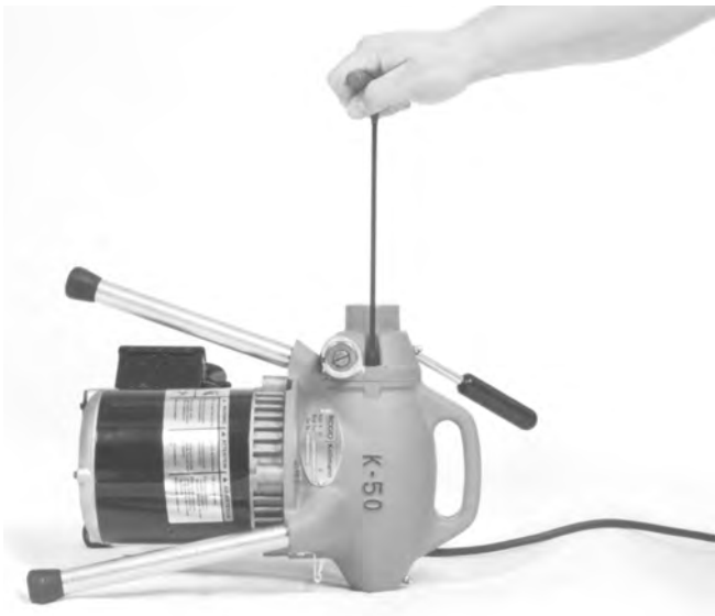
Figure 10 – Remove Socket Head Cap Screws
