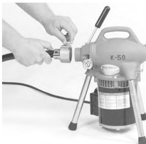
Figure 2 – Rear Guide Hose Attachment
