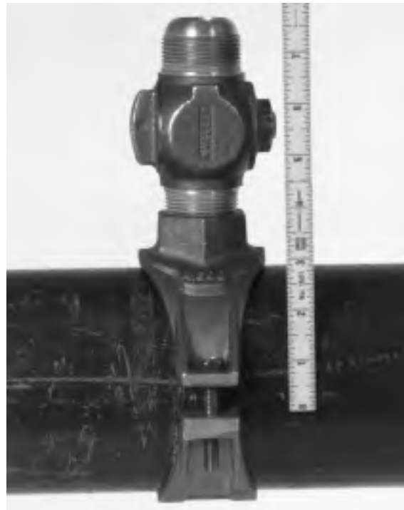
Figure 9 – Measuring valve standoff distance
