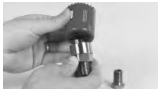
Figure 4a – Installation of cutter on large hole saw arbor
