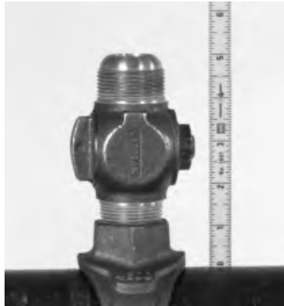
Figure 8 – Measuring valve standoff distance
