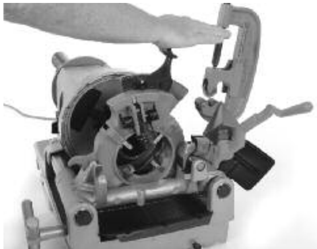
Figure 19 – Closing the Receding Die Head
