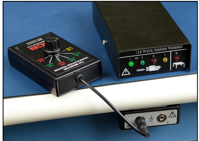
Figure 2. Using the 724VK2 Verification Tester with the 724 Workstation Monitor
