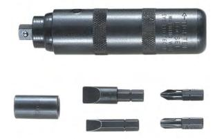
Klein Tools' Reversible Impact-Driver Set is a rugged, hand-impact driver designed to turn rusted, frozen, or other stubborn screws. The internal, spring-loaded, helical design transforms the impact of a hammer blow up to 200 ft. - lbs. of shock torque. It can also be used with 3/8-lnch square-drive impact sockets.
