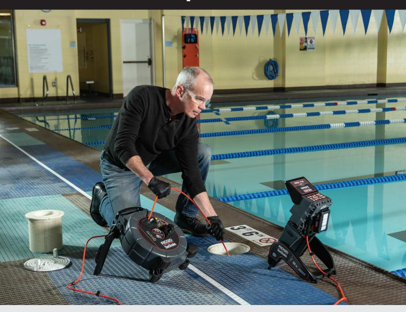
The RIDGID® SeeSnake® NANOreel® opens up new possibilities in drain inspection with the smallest-diameter camera and most flexible push cable of all SeeSnake® systems. Inspect a wide array of specialty applications that previously only bore scopes could reach.
