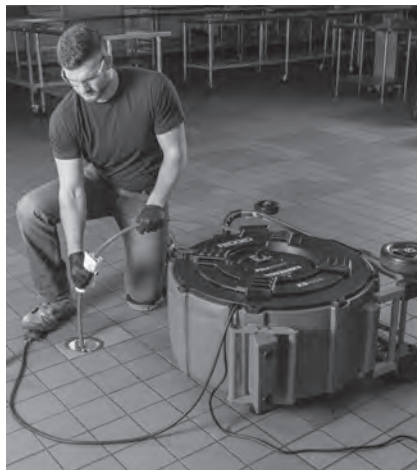
Figure 9 – Applying Lubricant to the Cable Sheath
