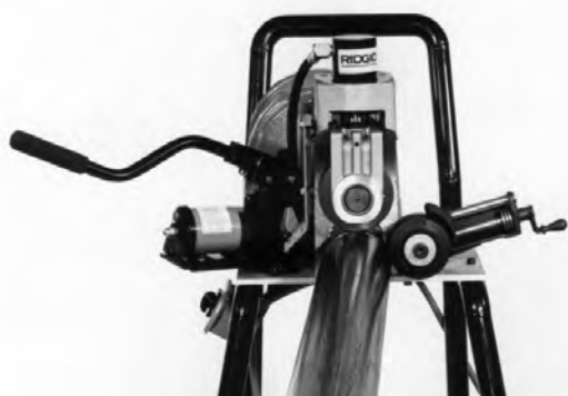
Figure 7 – Offset Pipe on 918-I (exaggerated for clarity)
