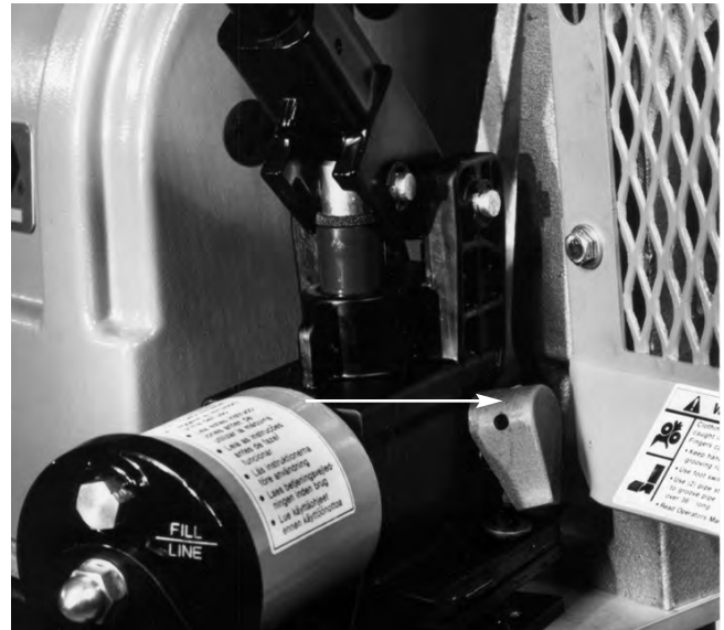
Figure 4 – Close-up of Release Lever on 918-I Pump
