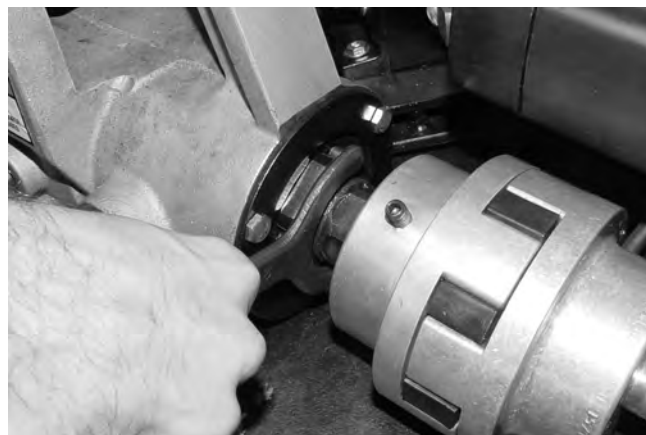
Figure 14 – Loosen and Remove Drive Shaft Retaining Nut
