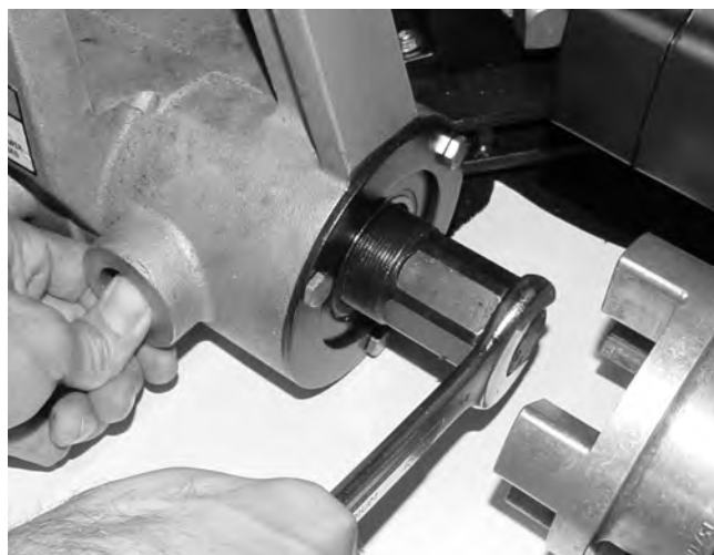
Figure 17 – Engaging Spindle Lock and Loosen Draw Bolt
