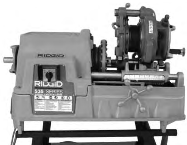
Figure 17 – Geared Threader Close-Coupled To 535
