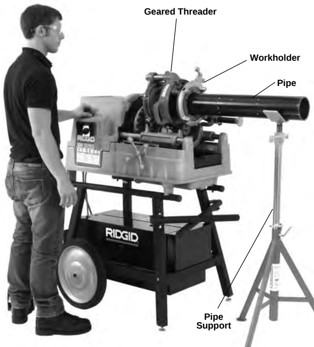
Figure 21 – Operating Position (Close-Coupled Method)
