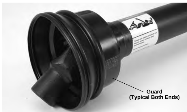
Figure 9 – 840A Driveshaft Guard and Warning
