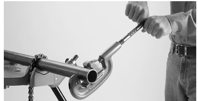
Figure 3 – Cutting End Of Pipe
