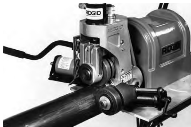
Figure 10 – Adjusting Pipe Stabilizer
