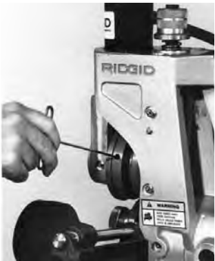
Figure 11 – Loosen Set Screw in Groove Roll
