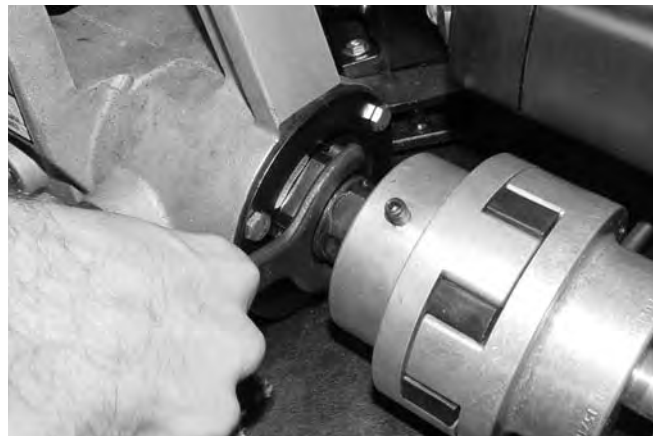
Figure 14 – Loosen and Remove Drive Shaft Retaining Nut
