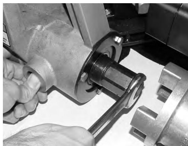
Figure 17 – Engaging Spindle Lock and Loosen Draw Bolt
