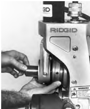
Figure 12 – Remove Groove Roll Shaft and Groove Roll
