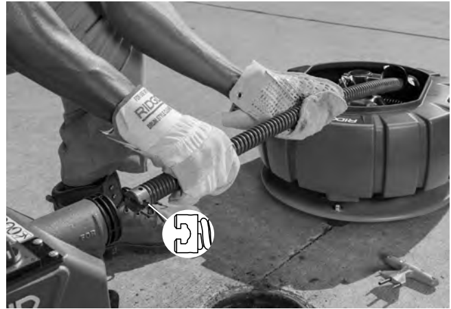
Figure 7 – Inserting Cable Into Front Of Machine
