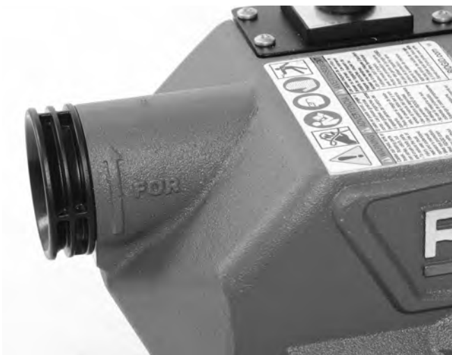
Figure 10 – FOR Machine Rotation Marking
